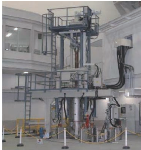
b. 电渣重熔炉 (3t, 铸锭直径600mm)
